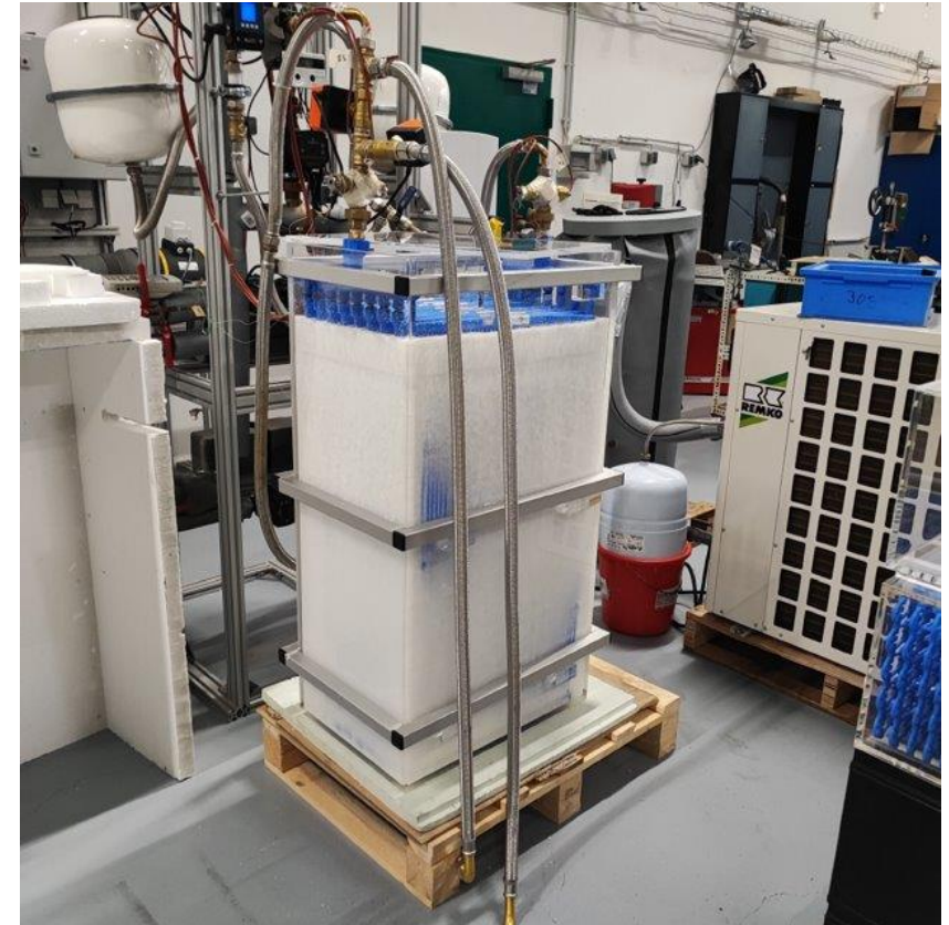
200 L storage filled with SP31 - Rubitherm
